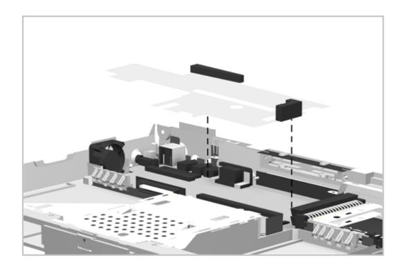
Figure 5-56. Removing the System Board Insulator
